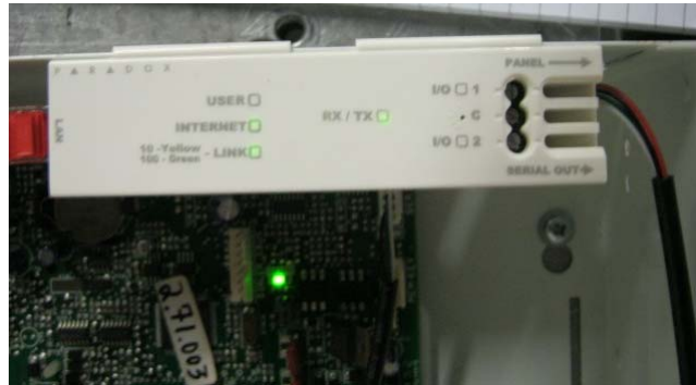
IP150 Mounted in metal Enclosure
